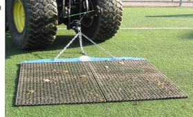
2 Start driving and brush for a couple meters. Maintain a maximum driving speed of 10 km/h.
