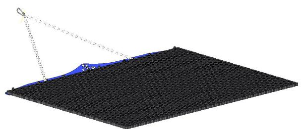
The Topfinish is connected to the tractor by a drag chain. This makes the tow mat suitable for any towing vehicle.
