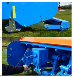
3 Stop aerating, lift the machine and turn it off;
